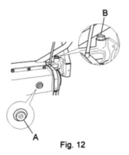
The oil should be replaced after the first 20 hours of use and after this every 100 working hours.
