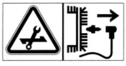
Warning. Always disconnect the cable from the engine spark plug.
