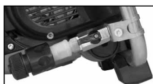
water supply opened (valve lever parallel)
